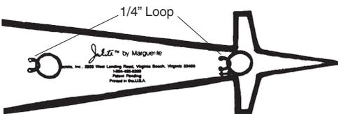
**STEP 8:** Bend white wires in half and slip on rings. Insert wires into aligning holes of back brace (from text side). Twist wire on inside of body. Do not tighten ring against the back brace, but allow 1/4" of space between the kite and the ring for the ring to move freely (this allows free movement of ring and controls wing flap).
