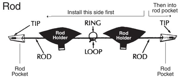
**STEP 10:** Press rod tips on end of fiberglass rod. Insert rod through rod holder, then ring, through rod holder and into rod pocket. Install rod into final rod pocket. ***The staples are critical and should exert no pressure on the rod which must be free to flex and move left and right.***
