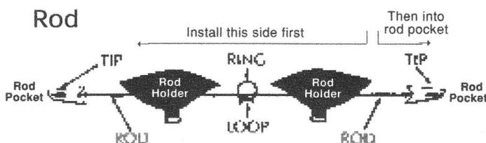
**STEP 3:** Insert rod under rod holder, thru ring, under rod holder and into pocket. Then install other end of rod into other pocket. Aft ring is not used for flight.
