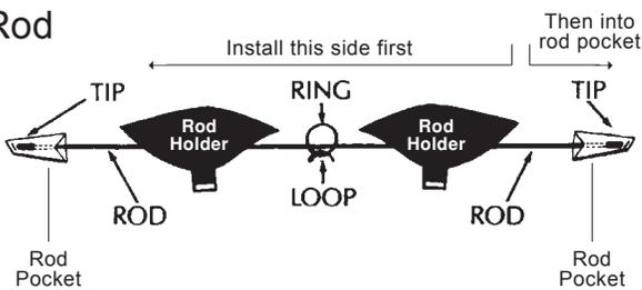
**STEP 11:** Press rod tips on end of fiberglass rod. Insert rod through rod holder, then ring, through rod holder and into rod pocket. Install rod into final rod pocket. ***The staples are critical and should exert no pressure on the rod which must be free to flex and move left and right.***
