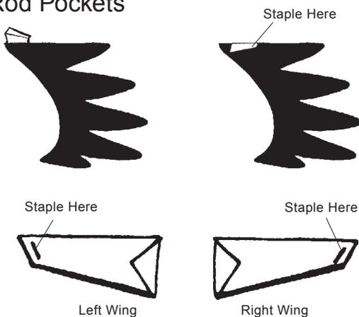
**STEP 4:** Form each rod pocket by folding on two score lines. Apply glue to shaded area and fold over onto the glued wing tip brace (pocket will be rounded). Staple or sew on white line 1/8" from pocket end.
