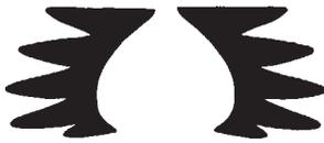
**STEP 2:** Apply glue to entire shaded side of each wing tip brace, and glue braces to wing tips (side with white area).
