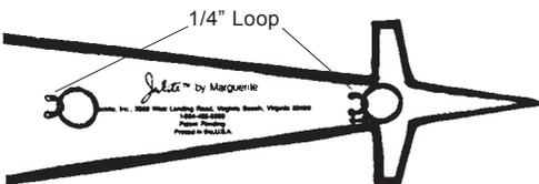
**STEP 8:** Bend white wires in half and slip on rings. Insert wires into aligning holes of back brace (from text side). Twist wire on inside of body. Do not tighten ring against the back brace, but allow 1/4" of space between the kite and the ring for the ring to move freely (this allows free movement of ring and controls wing flap).
