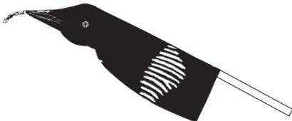
Insert one end of slat through body and into beak. Tape the other end down inside the body. This slat reinforcement keeps the head from bending in the wind.
